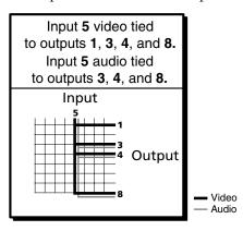
Figure 3-16 — Example 2, final configuration
